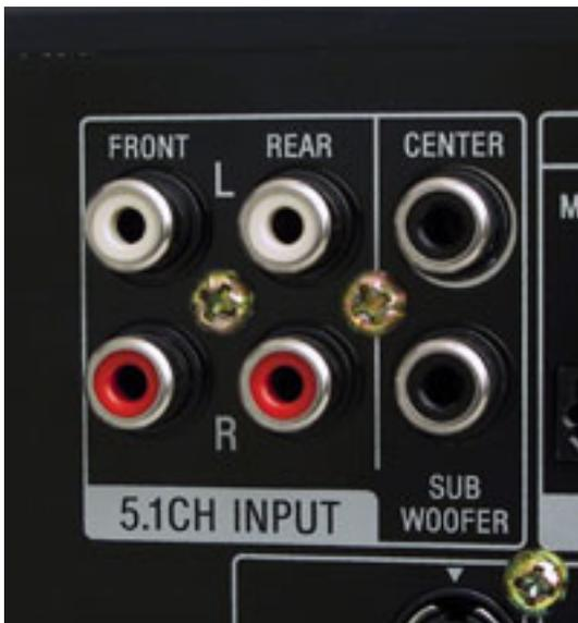
If your DVD player has the capability of playing back high-res DVD-Audio or SACDs, use this six-cable RCA connector set to connect to the analog multichannel input of the A/V receiver.
