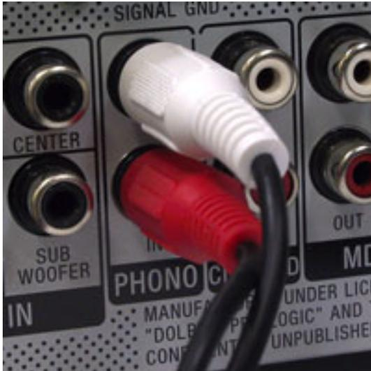
Always an RCA connection on A/V receivers or preamplifiers for the output from a turntable's moving-magnet (MM) or moving-coil (MC) phono cartridge. Still available on up-market receivers and preamps. Don't confuse this with "Phone Plug" (or Jack), which is a larger and sturdier ¼-inch diameter connector used on consumer A/V equipment for headphones.
